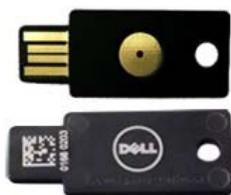
To generate a one-time password (OTP), touch the metal button on your YubiKey. The OTP is automatically entered at the current cursor position.
