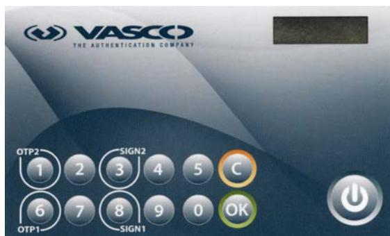
To authenticate and access resources protected by Defender, use the one-time password (OTP) application of the DIGIPASS 280 token (the OTP1 and OTP2 buttons). Currently, Defender does not support the e-signature application of the token (the SIGN1 and SIGN2 buttons).
