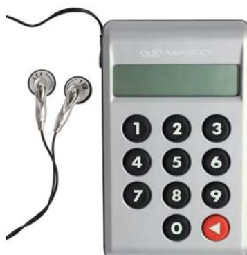
The DIGIPASS 301 CV is designed specifically for visually impaired people. This hardware token has an internal speaker and can be used with headphones attached.
